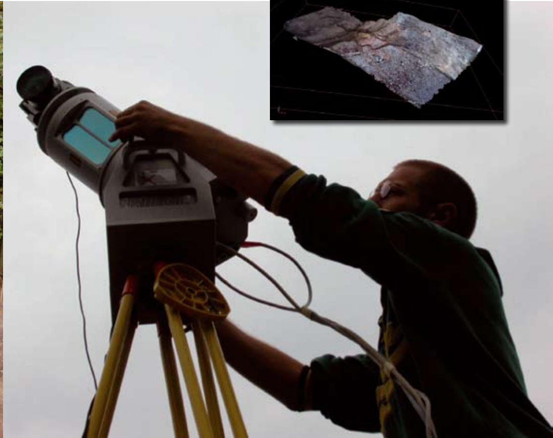
Arranging the 3D Laser Scanner for the record of complex surfaces uncovered during the excavation of the Iron Age workshops at Schwarzenbach-Burg.
