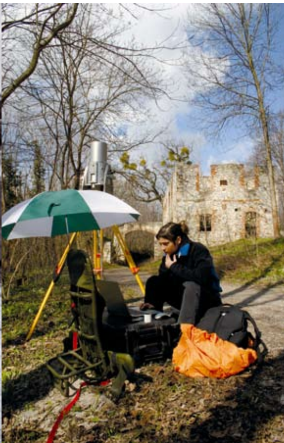
3D scanning of historical buildings at St. Anna in der Wüste, Austria.
