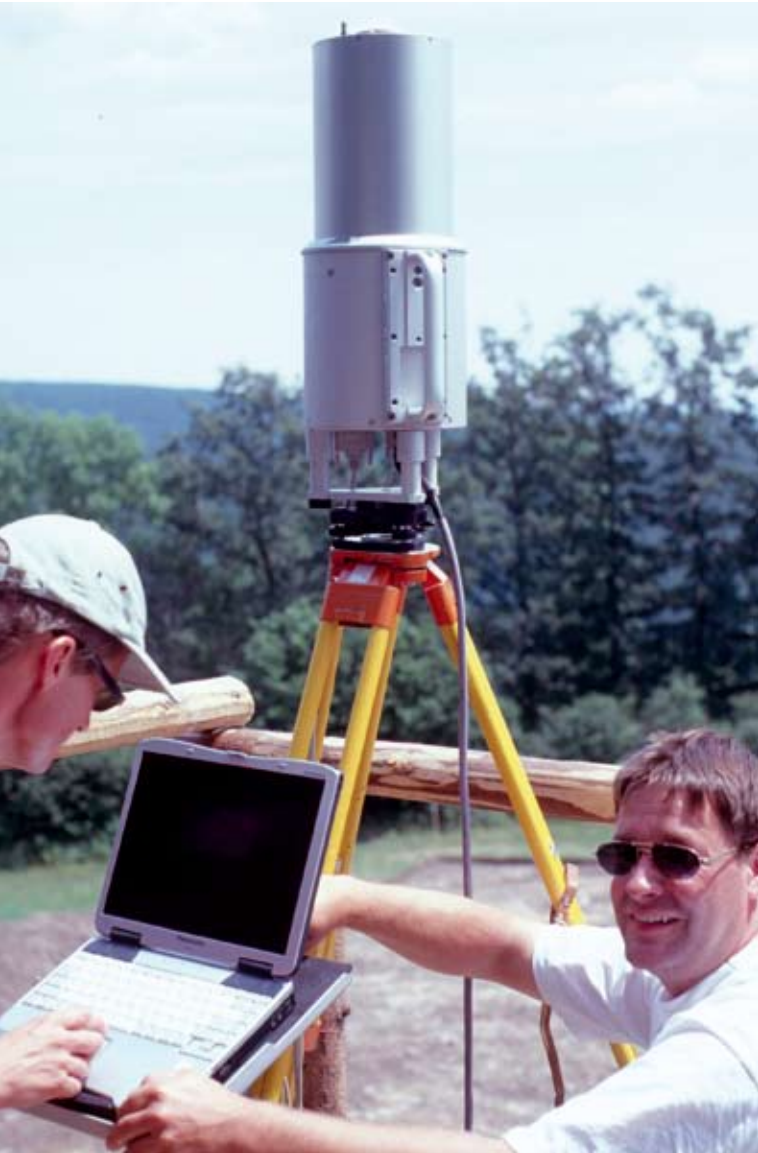
3D Laser Scanner Riegl LMS Z210 as first in use in Schwarzenbach in 2002.
