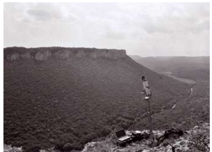
3D Laser Scanner Riegl LMS Z420i overlooking a valley on Crimea, Ukraine.
