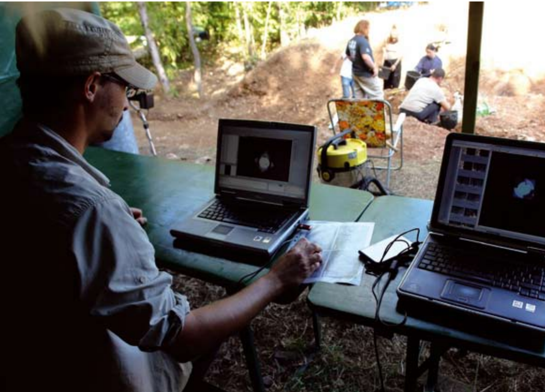
The recording Laser Scanner is controlled remotely via a WLAN set-up on site. Additional vertical photographs complete the photographic record.
