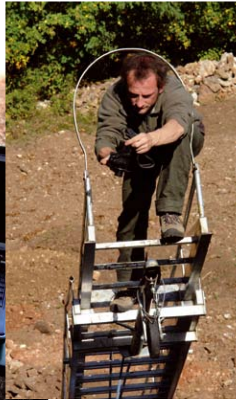
The recording Laser Scanner is controlled remotely via a WLAN set-up on site. Additional vertical photographs complete the photographic record.
