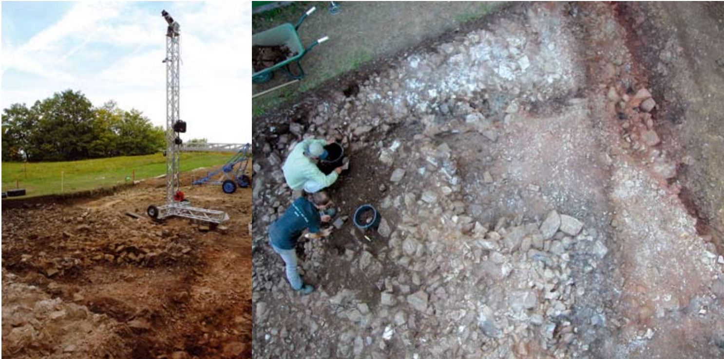
3D Laser Scanner Riegl LMS Z420i on a mobile scanning platform (MSP 250) in use to document the remains of the Iron Age workshops at Schwarzenbach-Burg.
