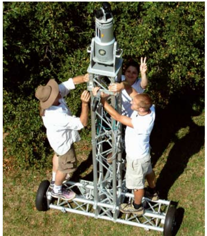
The documentation of the uncovered surfaces is done by 3D Laser Scanner combined with a digital camera.
